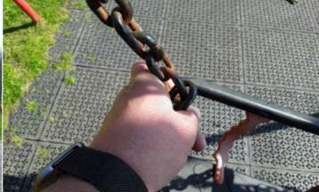
**Finding:** The chain links are worn in excess of 40% and require renewing
