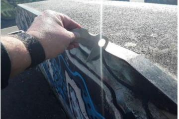
radius of less than 3mm and fails the requirements of BS EN 14974
