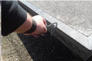
**Finding:** The item has exposed edges and corners with a radius of less than 3mm and fails the requirements of BS EN 14974
