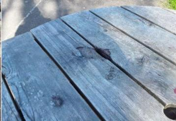
**Finding:** There is some evidence of fire damage to the item **Action:** Monitor for any further deterioration and repair as required
